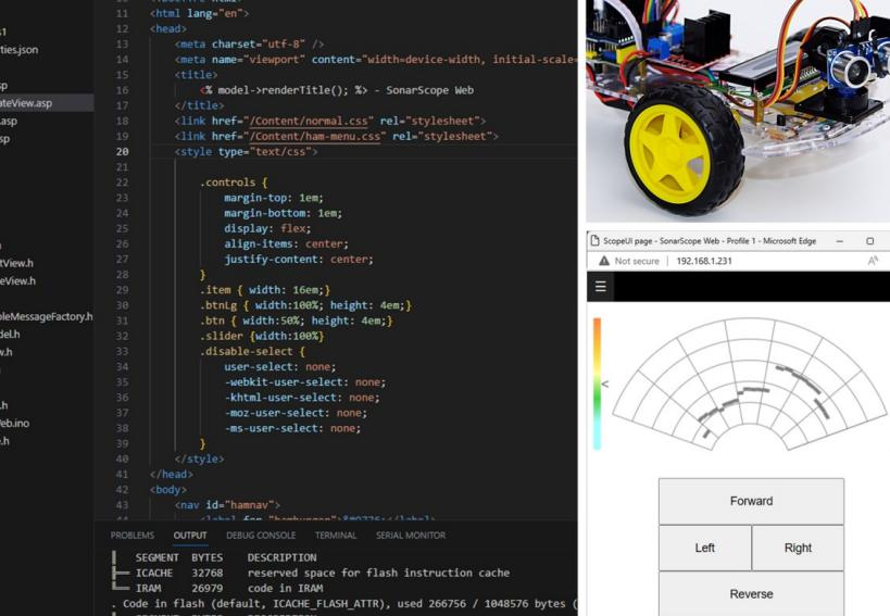
The screenshot shows the Visual Studio Code interface with the SonarScope\_Web project open. The Explorer sidebar lists files such as Arduino.h, BuildViews.pst, and various .h and .aspx files. The main editor displays the LayoutTemplateView.aspx file, which contains HTML and CSS code for a gauge chart. The CSS includes styles for controls, items, buttons, and sliders. The bottom status bar indicates memory usage (SEGMENT, BYTES, DESCRIPTION) and the Atmel STK500 development board.
